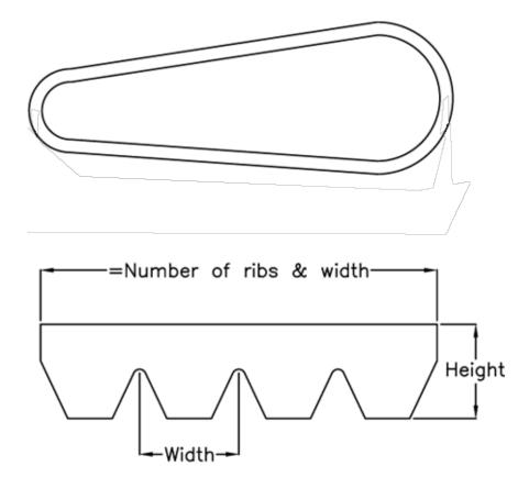
$\begin{aligned} \text{Datum Llength} &= 1300 \\ \text{Height} &= 3.5 \\ \text{Number of ribs} &= 20 \\ \text{Pitch} &= 2.34 \end{aligned}$
